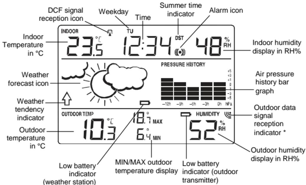
\* When the signal is successfully received by the weather station, the outdoor transmission icon will be switched on. (If not successful, the icon will not be shown on LCD). The user can then easily see whether the last reception was successful (icon on) or not (icon off).
