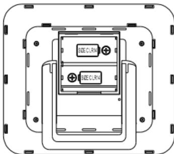
1. Remove the battery cover by sliding the battery cover upwards.
