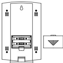
The Temperature Station uses 2 x AA, IEC LR6, 1.5V batteries. When batteries need to be replaced, the battery symbol will appear on the LCD. To install and replace the batteries, please follow the steps below:
