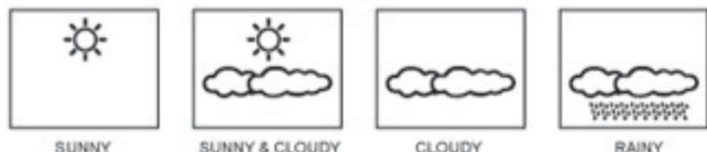
Your weather forecaster also has weather tendency indicator, when the air pressure is going up (the weather will improve) the UP arrow will appear, when the air pressure is going down (the weather will go worse) the DOWN arrow will appear.
