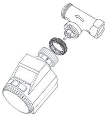
The energy-saving controller can only be installed if "INS" is showing on the display. Following installation, the actuator will perform an adjustment run so that it can adapt to the valve. During this process, "ADA" will be displayed.
