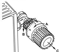
An adapter will need to be used in the case of certain valves. Adapters for Danfoss valves (RA, RAV, RAVL) are included in the scope of delivery. For details, please refer to the adapter overview (see 18).
