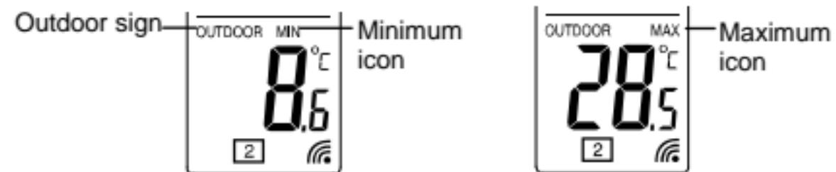
By pressing the “**MIN/MAX**” key the current indoor and outdoor temperature will alternate between the minimum, maximum and current temperature recordings. The time when the minimum and maximum outdoor temperature records were received will be also shown on the LCD blinking (recorded time is for outdoor temperature only). Once a new outdoor temperature high or is low reached, it will automatically be set into the Temperature Station’s memory.
