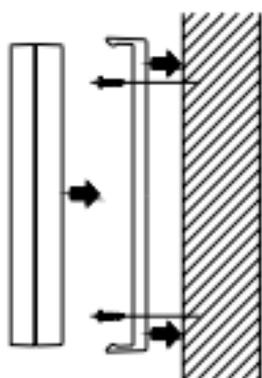
1. Mark the wall using a pen through the holes in the holder to obtain the exact drilling position.
