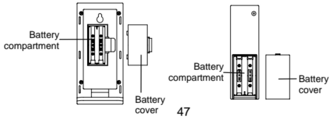
1. Flip open the battery cover at the back of the Temperature Station as indicated above.
