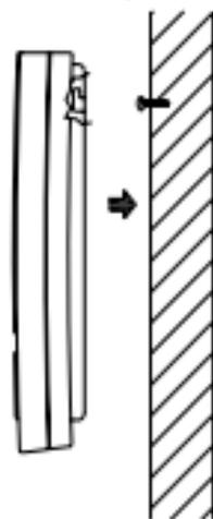
1. Fix a screw into the desired wall, leaving the head extended out the by about 5mm.
