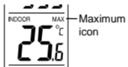
By pressing the “**MIN/MAX**” key the current indoor temperature will alternate between the minimum, maximum and current temperature recordings (also changes for outdoor temperature). Once a new indoor temperature high or low is reached, it will automatically set into the Temperature Station’s memory.
