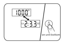
Press **g/LB** button (on unit bottom) to convert between metric and imperial units.
