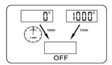
Auto switch-off occurs if display show **0** for 1 minute or shows the same weight reading for 1 minute.
