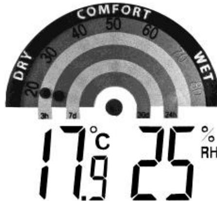
After starting up the device, it takes times in accordance with the interval until an average humidity value is displayed. Before the first average value the point on the scale is flashing slowly at 50%, in the app "---" is displayed.
