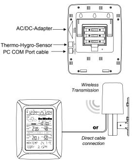
The direct cable connection of Thermo-Hygro Sensor and Base Station can be used in case that:
